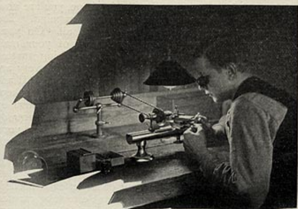
FIG. 4—FINEST JEWELERS' LATHES USED IN MACHINING NEEDLE VALVES
